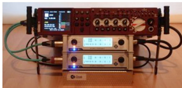
Figure 11: My Nagra VI with a pair of Neumann DMI-2 Portable for four AES42 microphones powered and clocked from the recorder
