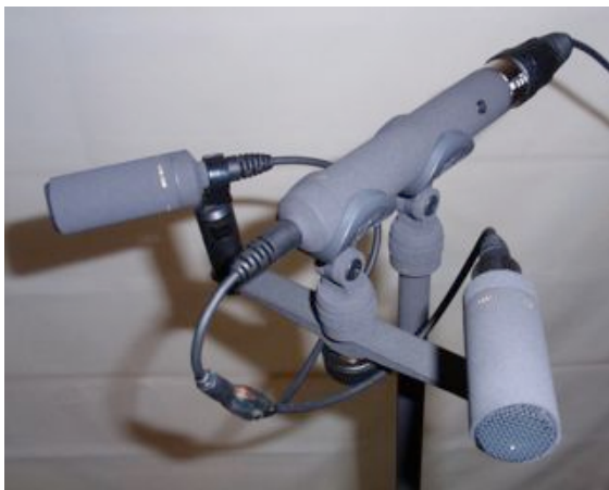
Figure 8: My Sennheiser MZD 8000 set-up with custom Y-cable and MKH 8020 stereoset
