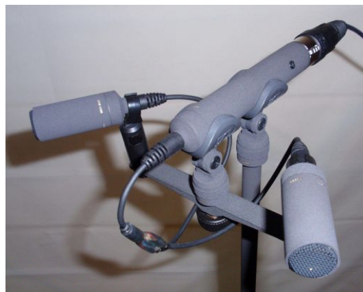
Figure 10 – My Sennheiser MZD 8000 set-up with custom Y-cable and MKH 8020 stereoset
