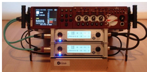
Figure 11 - Current rig: Nagra VI with a pair of Neumann DMI-2Portable for four AES42 microphones powered and clocked from the recorder
