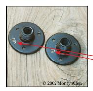
1. My podium mounts came pre-drilled with 3 holes, unfortunately they are wider than the clamp. You will need to drill one more hole per mount directly opposite of one of the pre drilled hole.
