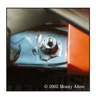
3. At this point you can attach the podium mount to the clamp with the bolts, lock washers and nuts. I travel a bit and the vibration in my car has known to loosen screws. These clamps are usually hanging over someones head, to play it safe I epoxy the nuts in place.
