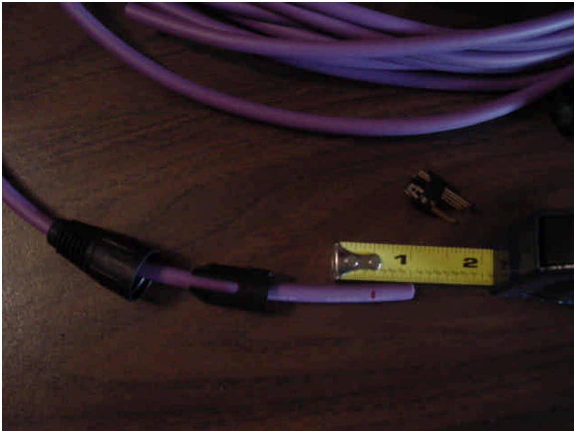
Image #2: Placing the connector & determining strip placement.
