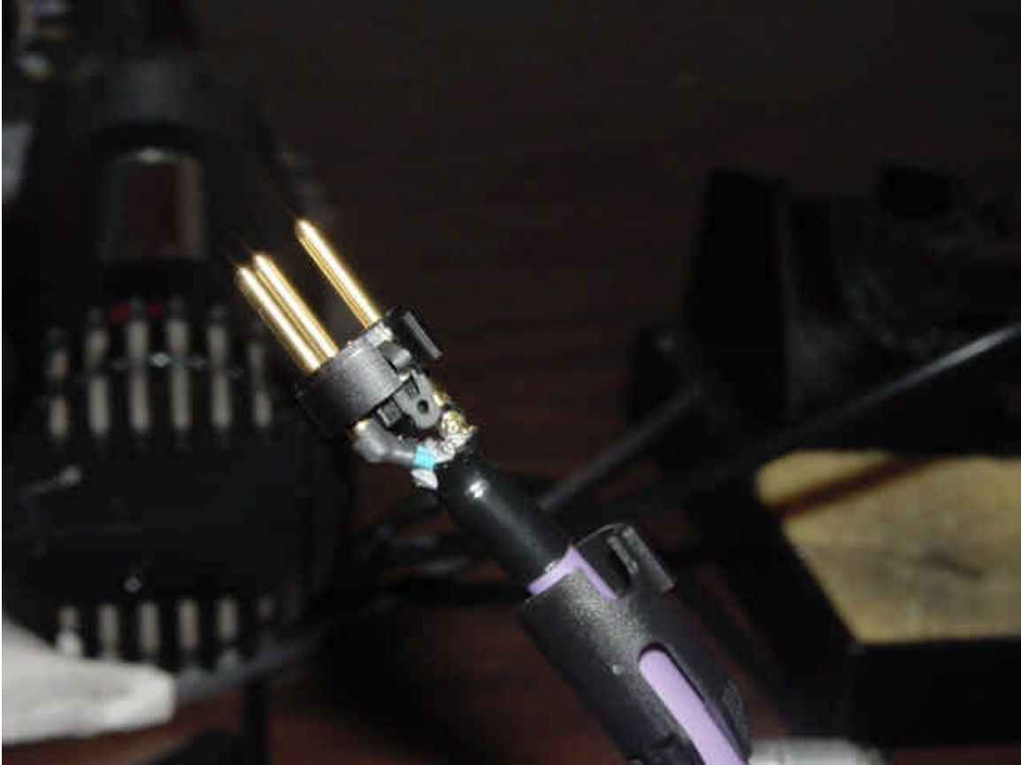
Image #6: All Pins soldered & heatshrinked to the Insert
