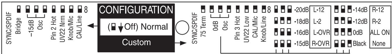
The black part of the DIP switches as indicated above represents the actuator of the switch. It may not be this color on the unit.
