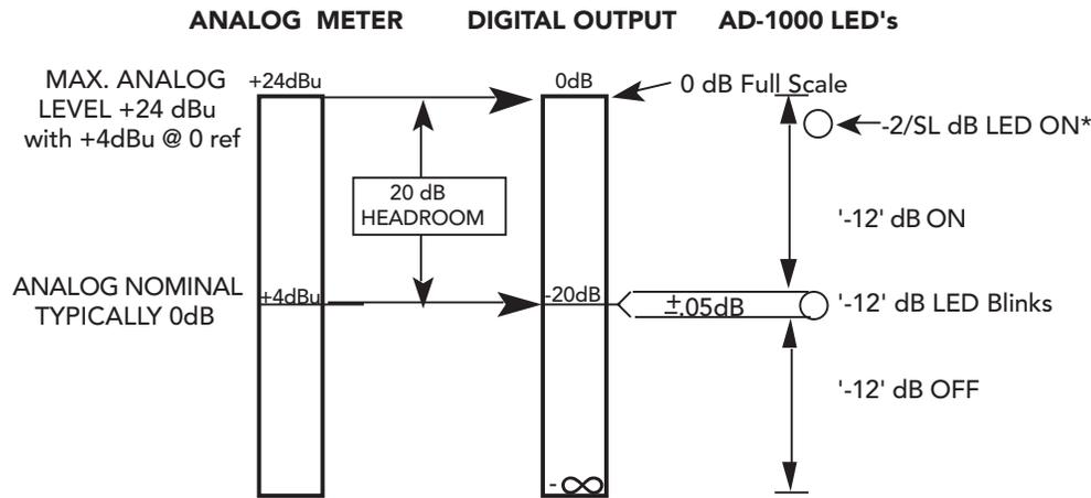
COMPARISON OF ANALOG INPUT TO DIGITAL OUTPUT WITH 20dB HEADROOM AND +4 dBu REFERENCE
