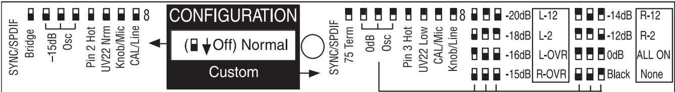
The black part of the DIP switches as indicated above represents the actuator of the switch. It may not be this color on the unit.
