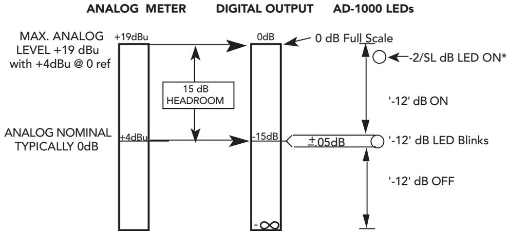
COMPARISON OF ANALOG INPUT TO DIGITAL OUTPUT WITH 15dB HEADROOM AND +4 dBu REFERENCE
