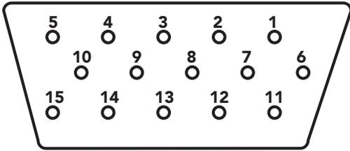
AD-1000 HD15 connector (J1) pin numbering viewed looking into the connector on the unit from the outside (numbers are as molded on the connector itself)
