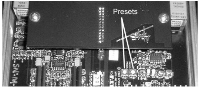
With these trim pots, you can adjust the ratio from 1:1 to 1:3. Each trim pot has the same range; the difference between the two compressors is in the time constant. With the trim pot turned counter clockwise all the way, the compressor ratio is 1:1 – essentially turned off. With the trim pot set all the way clockwise, the ratio is 1:3.
