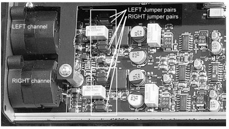
You will see four pairs of jumpers, two pairs for each channel. You can configure each channel independently if you wish, but be sure to move *all four jumpers for a channel*. The jumpers each plug on to three-pin connectors. Each jumper connects the frontmost and center pin for high gain (factory default) or the center and rearmost pin for reduced gain. To reposition a jumper, grasp it with a pair of tweezers and pull it directly upwards to remove it, then replace it over the desired pins.
