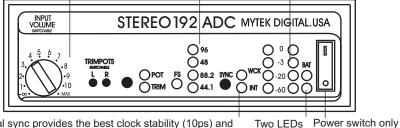
Internal sync provides the best clock stability (10ps) and thus the best conversion. External sync is intended for complex systems. It can be a standard wordclock signal or Protools (tm) 256X superclock. Refer to "Internal jumper settings" for details. Since internal clock generator is top notch, there is no sonic benefit from clocking Stereo192ADC externally. The ultra stable ADC clock however is a great clock to drive other digital equipment.
